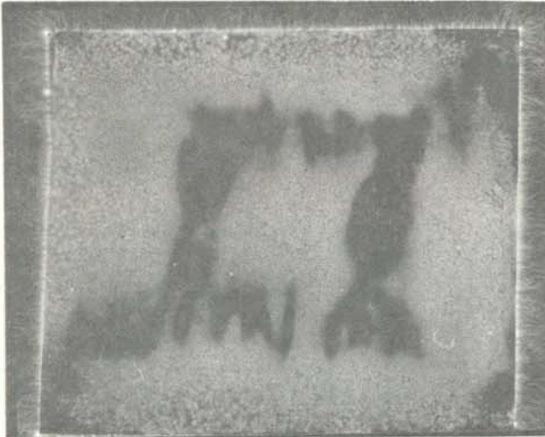
Figure 11 Photograph of Aquadag painted between two squares of aluminum foil and sandwich between two sheets of graphite paper. In all cases, the areas of graphite produce the same discharge pattern.
