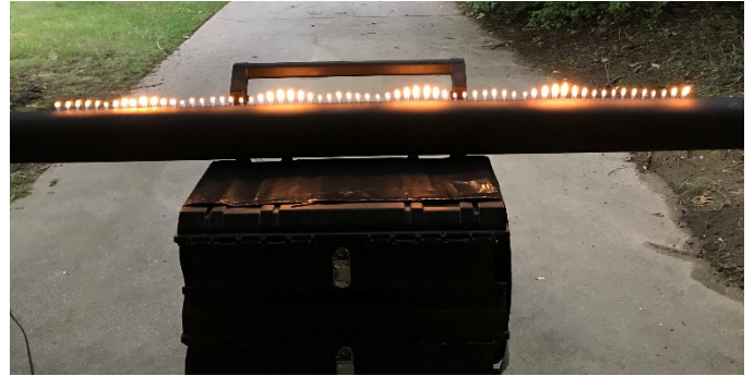
Make a flaming tube to explore the physics of acoustics and waves.
