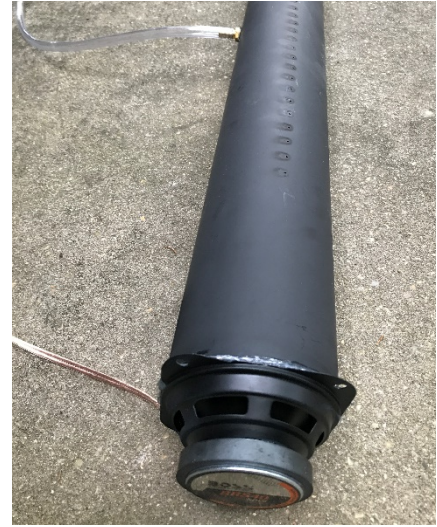
Figure 2 Speaker attached to end of tube. In this case, we kept the speaker attached to the tube with caulk.
