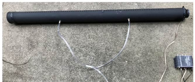
Figure 1 Joining the latex hose. The dual holes allow propane to get into the pipe quickly and evenly.
