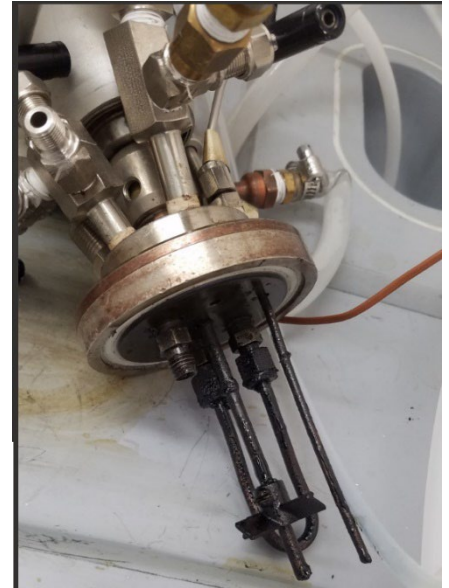
Images (Left to Right): 1) Assembled parr reactor, with pressure gage. 2) Mantle of the Parr reactor with crude biofuel inside (black slurry). 3) Cap of a Parr reactor with a stir bar and Temperature, Pressure sensors.
