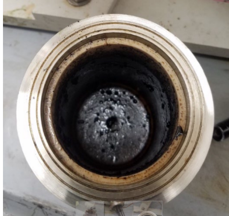
Images (Left to Right): 1) Assembled parr reactor, with pressure gage. 2) Mantle of the Parr reactor with crude biofuel inside (black slurry). 3) Cap of a Parr reactor with a stir bar and Temperature, Pressure sensors.
